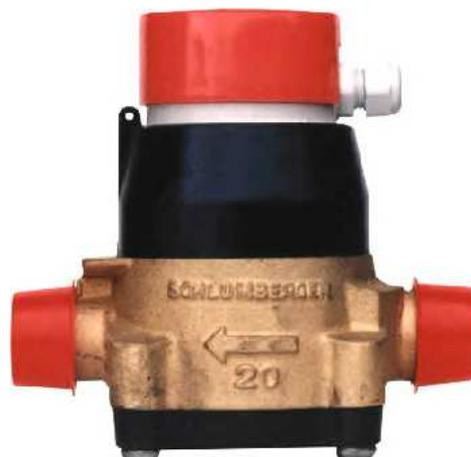
The FS-MES20, FS-MES25, FS-MES32 and FS-MES40 are magnetically coupled positive displacement pulse output flowmeters using the nutating disc measurement principle, providing a high resolution square wave transistor output or reed switch output.
