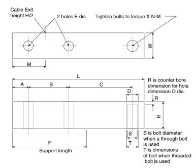
Capacities: 0-50kg to 0-10t Tool Steel Construction Electroless nickel plated
