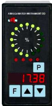
Circular graph and 5 digit display
