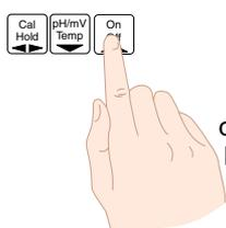
1. Remove power from the instrument using the On Off button. Hold in the Cal Hold button and switch on again by pressing the On Off button. The display will indicate **CAL** as part of the "wake up messages" when the **CAL** message is seen you can release the buttons.
