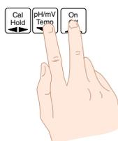
3. Within 2 seconds of releasing the Cal Hold button press, then release the On Off and pH/mV Temp buttons together. The display will now indicate **FUNC** followed by the first function.
