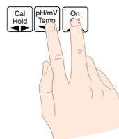
3. Within 2 seconds of releasing the Cal Hold button press, then release the On Off and pH/mV Temp buttons together. The display will now indicate **FUNC** followed by the first function.
