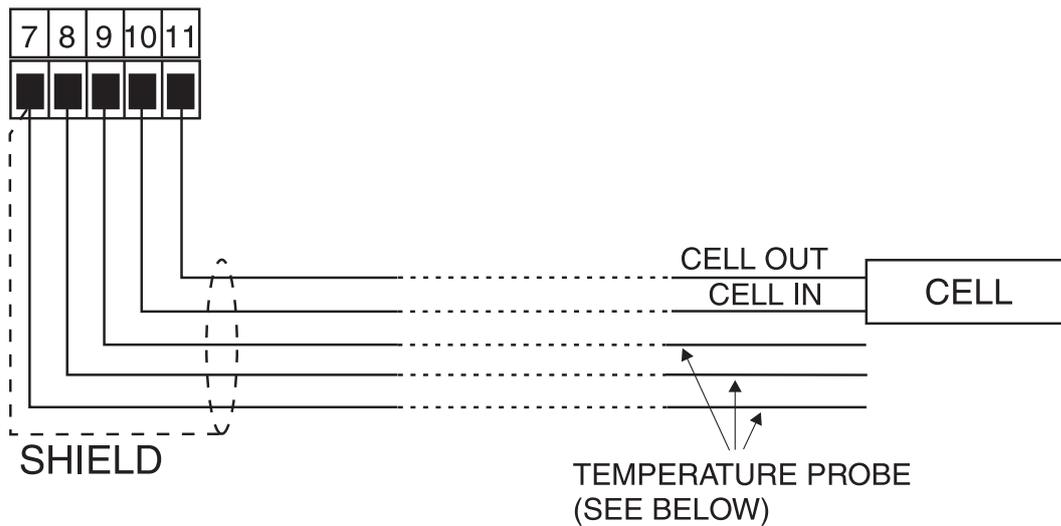
Temperature sensor - in most cases the temperature sensor is housed in the conductivity cell.
