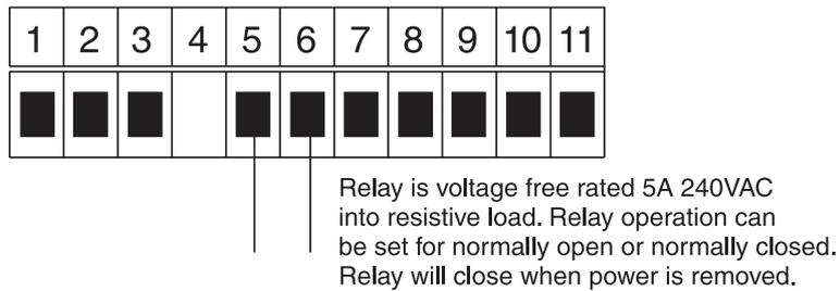
Conductivity and temperature wiring
