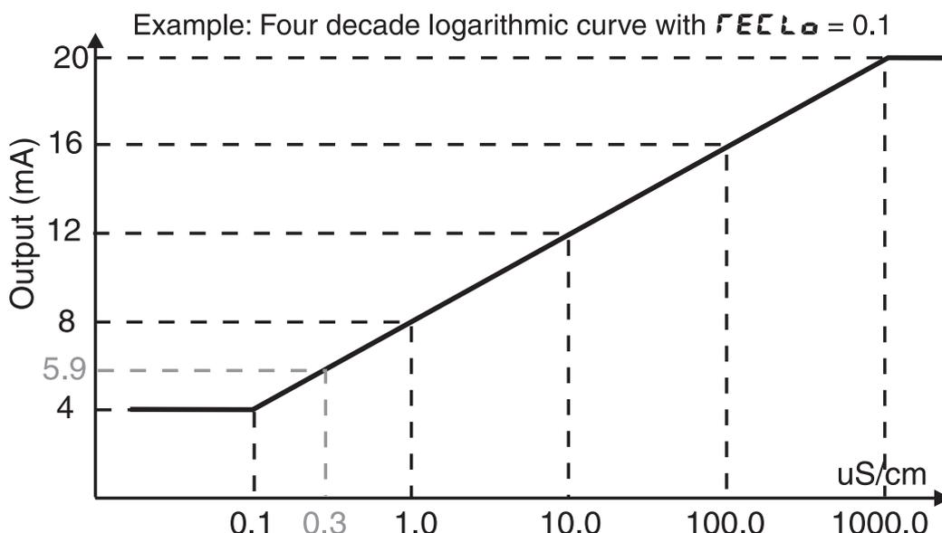
Example: The first decade runs from 0.1 to 1.0uS/cm. Because there are 4 decades in this example this gives a change of 4mA per decade. If the reading of 0.1uS/cm gives an output of 4mA and the reading of 1.0 uS/cm gives an output of 8mA then a reading of 0.3uS/cm will give an output of 5.9mA calculated from:
