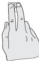
2. Within 2 seconds of releasing the **F** button press, then release the **▲** and **▼** buttons together. The display will now indicate **FUNC** followed by the first function.
