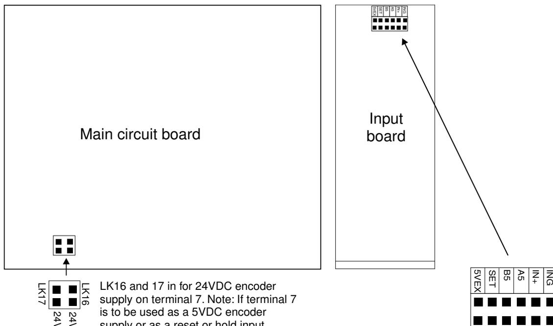
LK16 and 17 in for 24VDC encoder supply on terminal 7. Note: If terminal 7 is to be used as a 5VDC encoder supply or as a reset or hold input then LK16 and 17 must be out.
