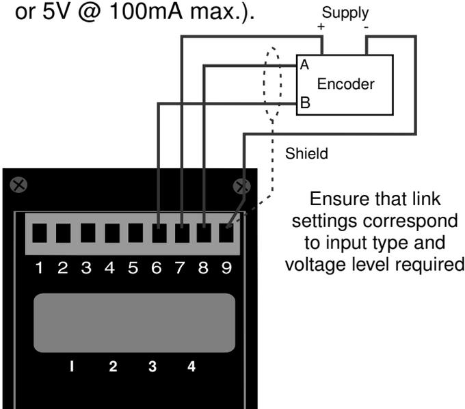
Encoder powered via optional 12 or 24V regulated (25mA max.).
