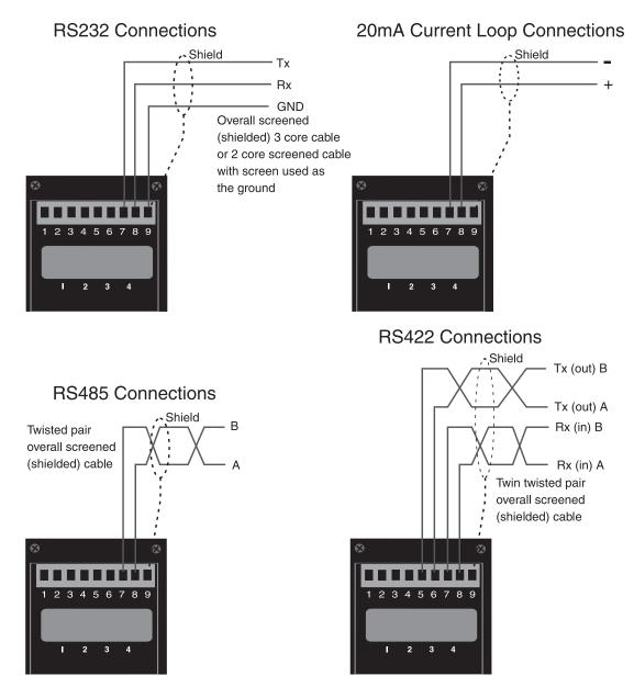
Note: the serial connections are isolated, therefore the screen should be connected to ground at both ends
