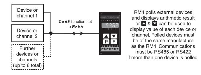
4. Scanning mode. Allows the RM4-RS to scan up to 8 inputs from other devices and display the value together with an indication of which input is being viewed. The input devices must be of the same manufacture as the RM4 and the serial communications must be via RS485. A special mode allows the RM4-RS to act as a slave display when connected to a model TP488 eight channel scanning monitor equipped with a serial output.
