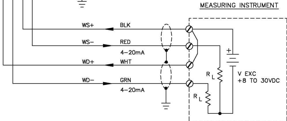
$$\text{MAX LOAD RESISTOR } (R_L) \text{ VALUE} = \frac{V_{\text{EXC}} - 10}{0.02} = R_L$$
