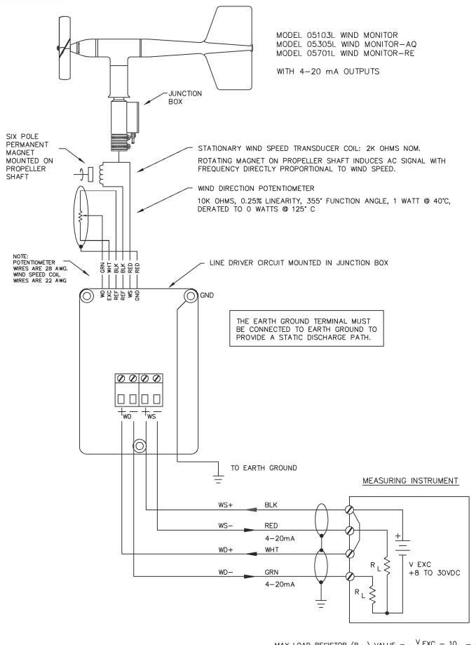
MAX LOAD RESISTOR (R  $_{L}$  ) VALUE =  $\frac{V \text{ EXC } - 10}{0.02}$  = R  $_{L}$
